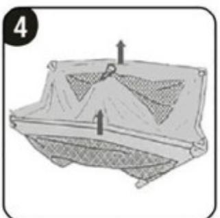
Lift the long-side rails until they lock into position.
