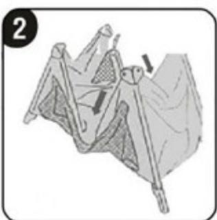
Lift the centre of the rails of the longest sides in the centre by squeezing the button underneath the top part of the rail & drop the rails down
